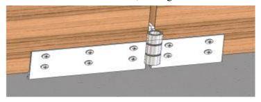
2. Slide the folding door rotating mechanism assembly from the side into the slot of the fixed bracket, install it to the leftmost side of the short bracket, and tighten the nuts at the upper and lower ends.
