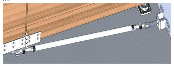
4. Test the folding effect of the door body, which can be adjusted by adjusting the length of the connection rod, the fixing base, etc.
