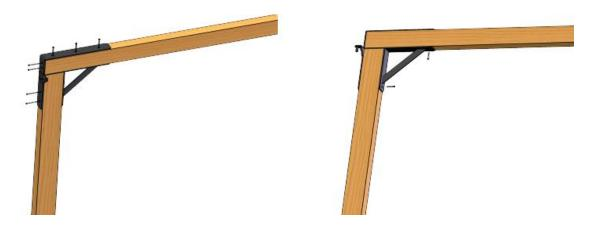
Step 3. Install the gate frame and tighten the screws.
