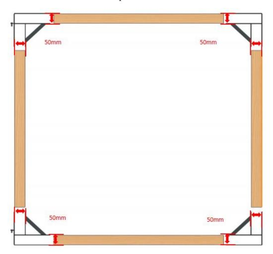
Step 2. Determine the position and tighten the flathead wood screws at the four brackets.
