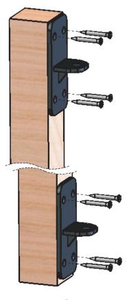
Step 5. Align the axes of the upper and bottom fixed inner brackets with the hinge holes on the gate post and install them.
