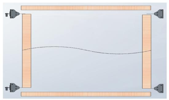
Step 2. Determine the position and tighten the flat head wood screws at the four brackets.
