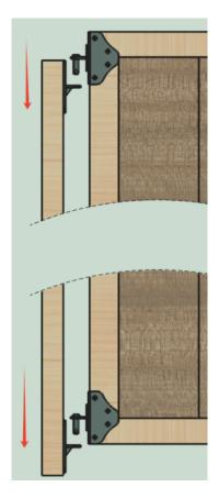
Step 6. Attach the gate latch kit to the inside gate post at the desired height use the round head wood screws.
