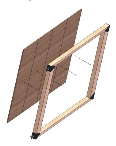
Step 4 . Measure the gate frame to determine the hinge height, and tighten the flat head wood screws to fixed the gate hinges on the gate post.
