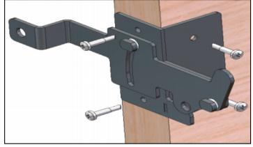
Step 7. We also provide a lock bracket (working with gate latch), if need, you can install it with round head wood screws on the gate so that users can add a lock.
