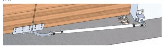
4. Test the folding effect of the door body, which can be adjusted by adjusting the length of the connection rod, the fixing base, etc.
