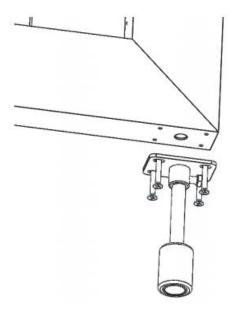
7. Fully closed the door, mark the position of the rubber stopper hole, and drill a hole with a  $\phi10$  drill bit.
