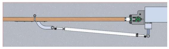
5. After adjusting the tightness and the door opening and closing effect, install the connection rod cover and base cover from the top.
