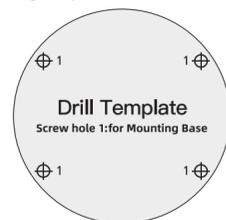
4.3 Drill the four holes and use a hammer to gently insert the anchors into the wall.
